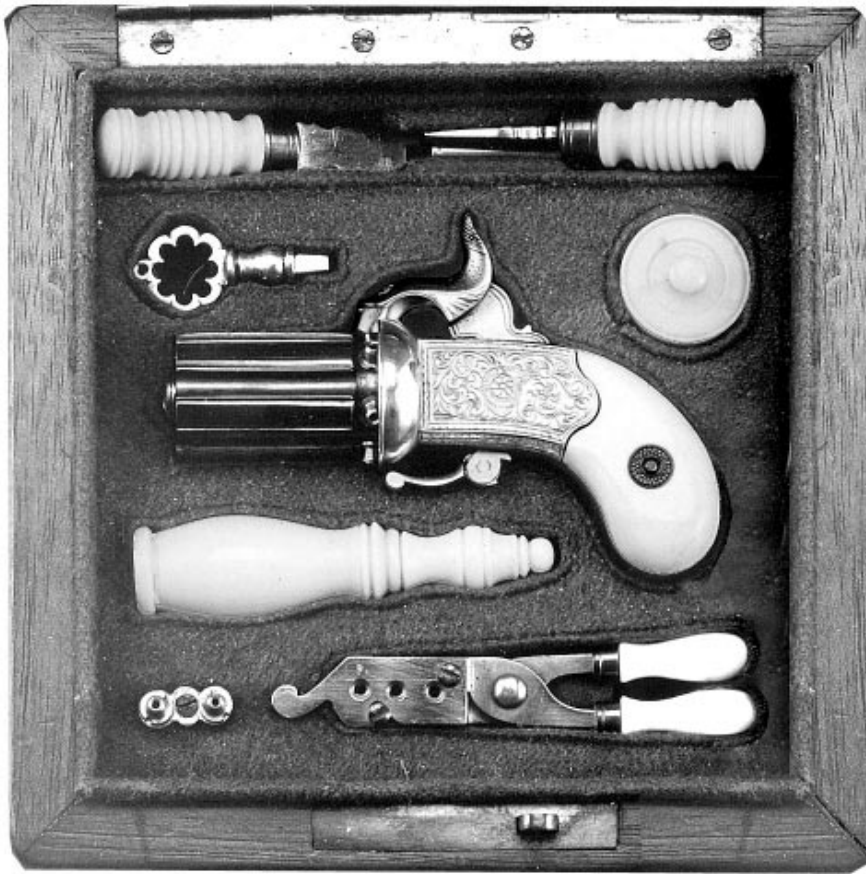
To the left is a cased 1/2 scale, six shot, pepperbox made by John Maycock. It has a blued barrel with Silver plated frame, and ivory grips. The case is loaded with every possible accessory including; a bullet mold, ivory powder flask, barrel wrench, screwdrivers, and percussion cap container.
