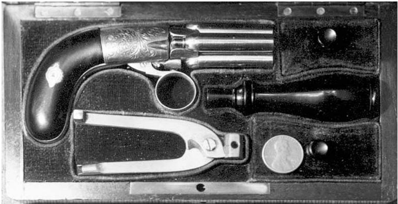
Below: Another fine, cased, engraved, (four barrel?) pepperbox of the Mariette design, with ring trigger, under-striker and wood grips.
