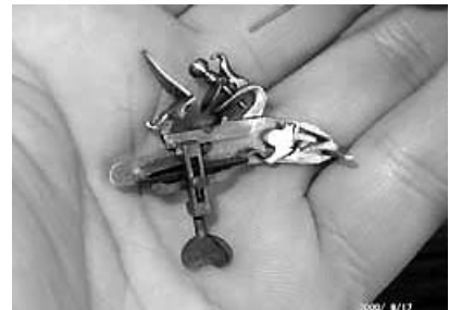
Right: The well used spring clamp from the 1/4 scale Turner Kirkland commemorative Kentucky Flintlock Pistol shown below. OAL is 2-3/4"
