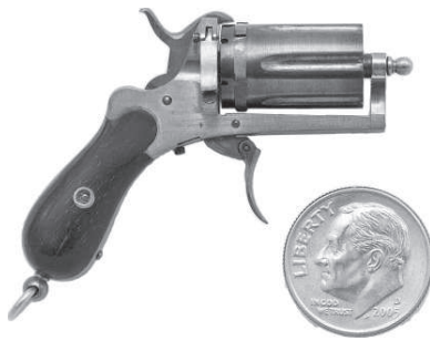
6.4mm French Pinfire Fist Pistol 6-shot Revolver; 1/3 scale, brass frame, blued cylinder hammer and trigger, ebony grips, Length: 1-3/4"
