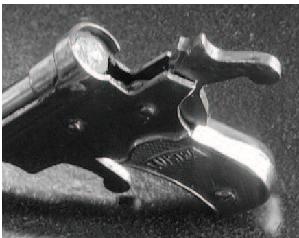
Above: we see the plugged barrel, and flattened firing pin on the hammer.
