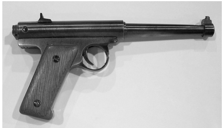
Above: A 1/2 scale Ruger profile mini that fires 2mm rimfire. This one was based on a Ron Dewalt design that Lew liked.
